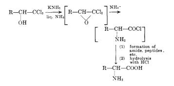
The conversion of four trichloromethylcarbinols to 'amino acids was studied (Table I). The R group in the above equation was ethyl, isopropyl, and phenyl. In addition, 1,1,1-trichloro-2-methyl-2-propanol (chlorobutanol) was studied. In all cases, the reaction was
